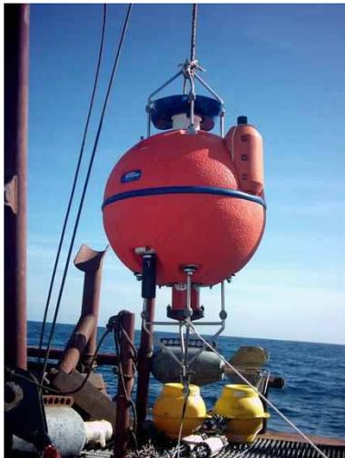
The scope of work called for current measurements at a single location in the centre of the Riyan prospect in water depth of  $\pm 660\text{m}$  for a period of up to 180 days. The mooring comprises a combination of 75kHz and 300kHz acoustic doppler current profilers (ADCPs) so as to be able to obtain a current profile through the entire water column.
