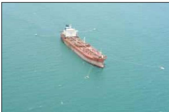
TEMA offshore imports petroleum products via a Conventional Buoy Mooring (CBM) system into Ghana (see picture on left). The existing system comprises an 18" pipeline between the CBM and Tema Oil Refinery.
