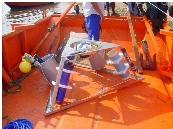
The AWAC system has been fitted with dual Sonardyne lightweight acoustic release transponders that will allow its recovery at 2 monthly intervals for data download and processing. A Seimac Novatech AS900A satellite locator beacons has also been fitted to the system to allow its location in the event that the system is recovered by a 3<sup>rd</sup> party.
