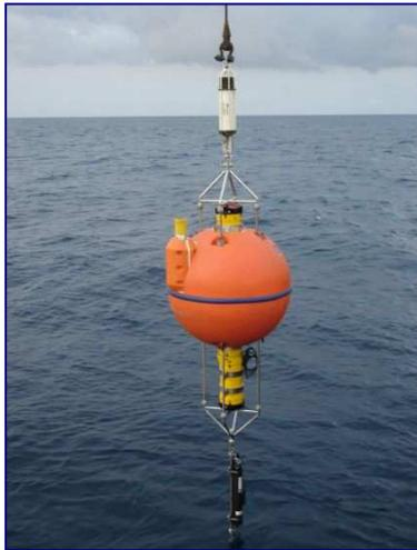
Deployment of the moorings was conducted from the Sonatide vessel Russell Tide (below right). Due to the high accuracy requirements in terms of mooring positioning, both moorings are fitted with Sonardyne mini transponder beacons and the channel mooring was lowered anchor first to the seabed using the vessel's A-frame and winch (pictured on left). Once on the seabed the mooring was inspected by ROV to ensure it was located in the centre of the channel.
