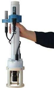
The unit supports both RS232 and RS485 data communications and external power, in addition to the standard internal autonomous mode.
